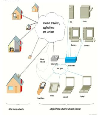
As we can see each and every Wi-Fi signals needs a Wi-Fi router to send and receive data. These routers are again connected by wires to the internet provider through a modem. Wi-Fi works with the help of radio waves and so far every device that gets connected to the internet we need to provide and additional piece of hardware that could send and receive RF signals.
